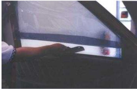
#19 (optional) Place a tool between rubber and glass. Any smooth flat tool can be used.
