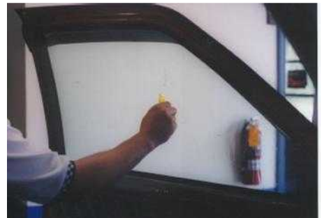
#22 Spray window again and squeegee the entire window again, starting at the top working down and toward the sides (do not roll window down, start as high on glass as possible)
